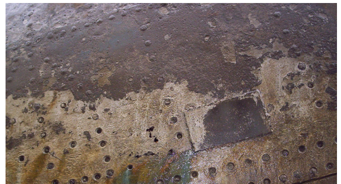
Photo showing missing rivet heads, entire rivets, and holes in the hull plate. Also shows the patch OMMF applied to stop the leak in after fuel tank on the port side.
