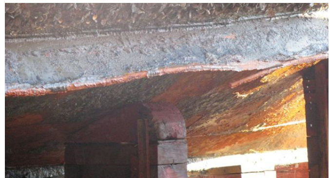
Damaged bilge keel on the port side.
