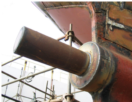
The can installed over the propeller shaft.
