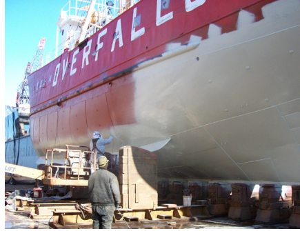
The second coat of paint on the new steel.
