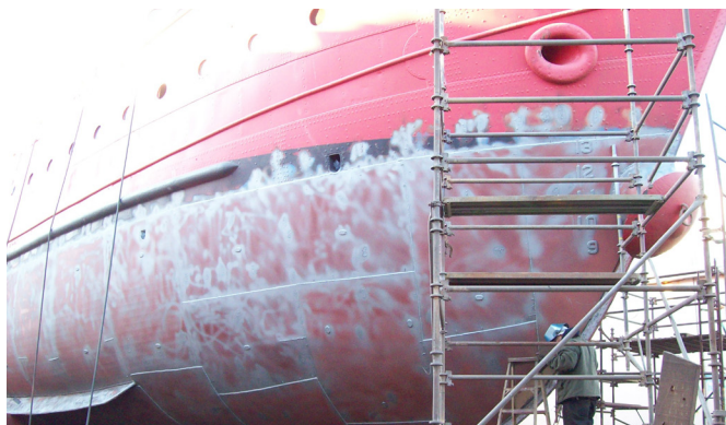
New steel plates installed, primed and ready for the first coat of paint.
