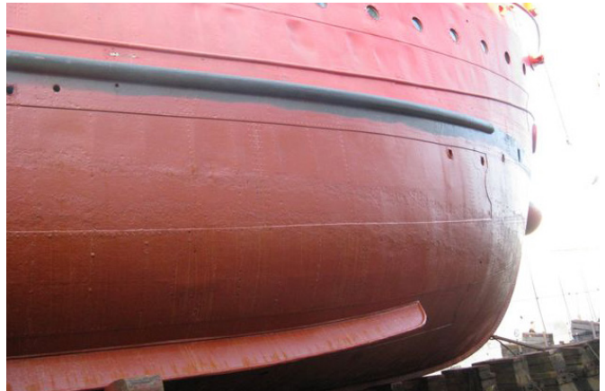
Old hull plate cleaned, painted and ready for new plates.
