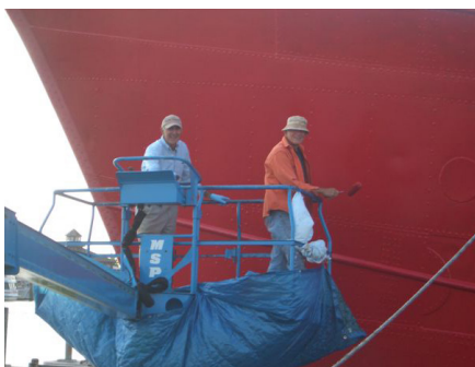
Top: Before and after painting the hull red (black bottom) before and after. Bottom: Painting the hull from platforms and aerial lift.
