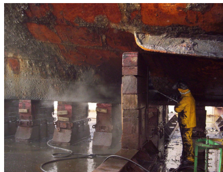
Washing the hull with 40,000 PSI pressure.
