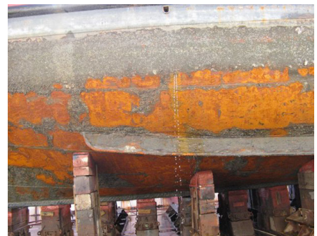
Water draining from the hole in the #4 fuel tank on the starboard side.
