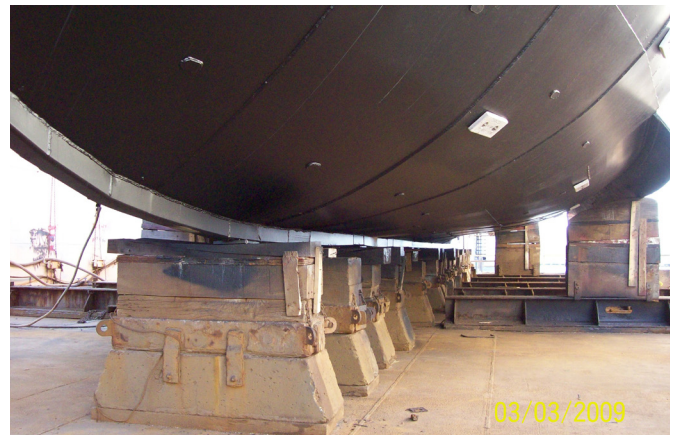
New keel bar channel runs the length of the ship.
