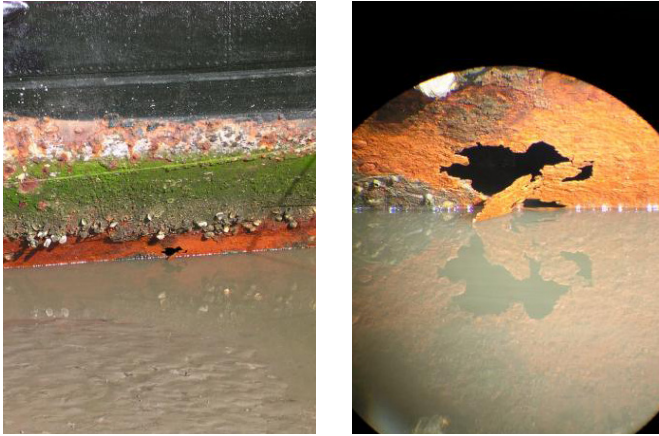
Left: Hole in the hull through to the shaft alley. Right: The same hole looking through a scope.
