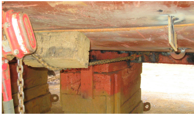
New hull plate being bent into shape for welding.
