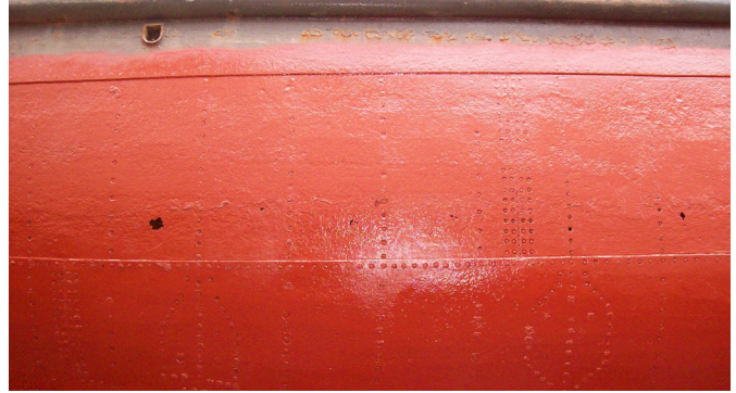
Hole in #4 fuel tank after cleaning and painting. (Note other holes and rivets)
