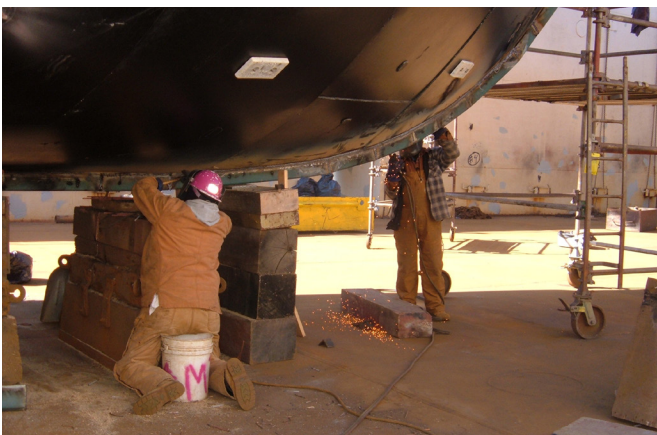
Installing the channel on the keel bar.
