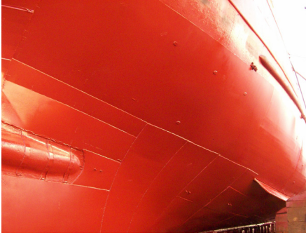
The first coat of paint on the new steel.
